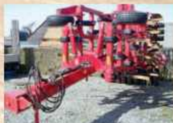
Horsch Tiger 4 AS Bj. 2010, 17 TerraGrip Zinken, Top Ring Packer, Bremsanlage
